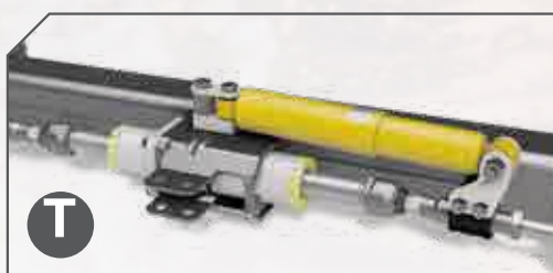
Possible mounting positions of the shock absorber
